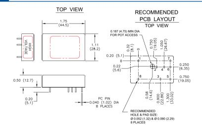
Description 5Vin 12Vin Pin Function VOUT High Voltage Output Ground to Pin 8 1 2 VPGM Voltage Programming Input, <150uA 0 to +2.048V 0 to +5V 3 SGND Signal Ground [For VPGM, VIN, VMON] Low Voltage Ground Voltage Reference Output, +/- 1% , 1 mA 4 VREF +2.048V +5V Case Ground 5 CGND Case Ground 6 VIN Input Voltage +4.75 to +5.25V +11.5V to +15.5V 7 VMON Voltage Monitor Output, 1mA, scales to 0 to 100% Vout 0 to +2.048V 0 to +5V 8 HV RTN HV Output Return Ground for Pin 1
