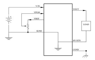
**Programming Voltage vs Output Voltage**
