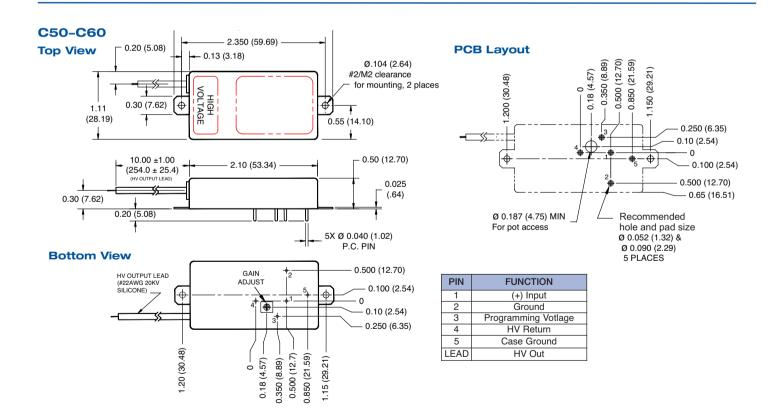
All dimensions are in inches (mm) Tolerance:  $X.XX \pm 0.02$  (0.51) Pin Tolerance:  $\pm 0.005$  (0.127) Weight: C25-C40: 1.3oz (36.8g) C50-C60: 1.8oz (51g)
