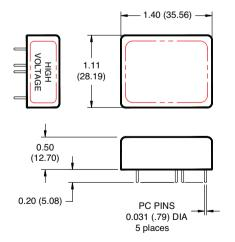
All dimensions are in inches (mm) Tolerance: X.XX  $\pm 0.02$  (0.51) Pin Tolerance:  $\pm 0.005$  (0.127) Weight: C01-C20: 1.1oz (31g)
