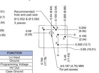
All grounds internally connected except case. Case ground (Pin5) must be connected to ground, with no more than 50V between case ground (Pin 5) and circuit ground (Pin 2).
