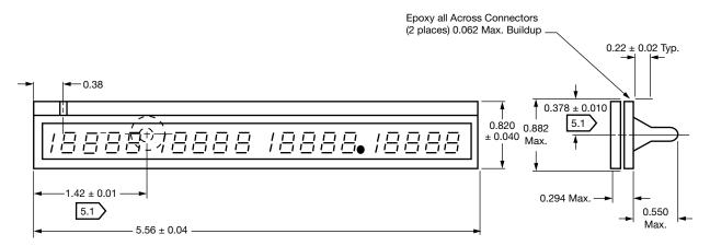
5.1 Fill tube is concentric with hole within ± 0.060 vertically and + 0.060/- 0.030 horizontally.
