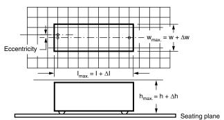
For the minimum product dimensions for length (I<sub>min.</sub>), width (w<sub>min.</sub>), and height (h<sub>min.</sub>) following tolerances of the components are valid:
