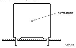
The temperature is measured in unloaded (T<sub>amb</sub>) and maximum loaded condition (T<sub>C</sub>).
