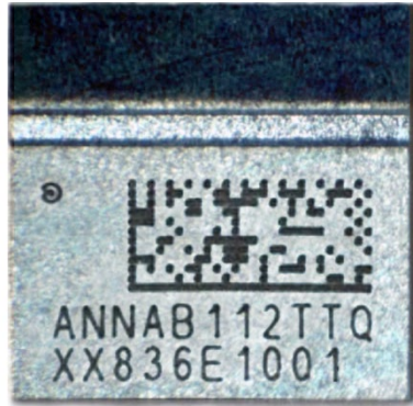
Figure 10: Product marking on the ANNA-B112 module
