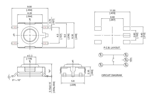
**Model SWTW-J** (Top Actuation, SMD J pin style, 6 x 6 mm)
