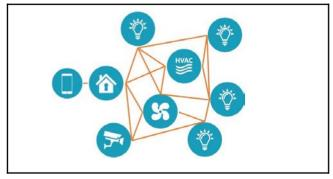
Mesh interconnected devices in a smart home network enable synergy effects e.g. by combining sensors such as light and temperature sensors with controllers for shutter, air conditioning, lighting and heating.
