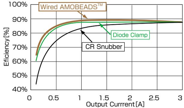
Power Supply Efficiency ( $V_{in}$ :DC 140V,  $V_o$ :24V)
