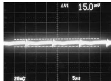
Wired AMOBEADS™ delay the turn-on time of the MOSFET when they are inserted between the gate of the MOSFET and drive winding on the primary side of the self-exciting single flyback (RCC). The wired AMOBEADS™ reduce both noise, due to surge current and switching loss, by turning on the switching element at the point when the voltage of the transformer becomes low, utilizing the LC resonance phenomenon induced by inductance L of the primary winding of the transformer and a snubber capacitor C.
