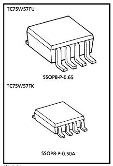
Weight SSOP8-P-0.65: 0.021g (typ.) SSOP8-P-0.50A: 0.01g (typ.)
