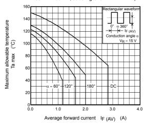
Ta max – I<sub>F (AV)</sub> Glass-epoxy substrate (substrate size: 50 mm  $\times$  50 mm, soldering land: 6 mm  $\times$  6 mm) 160 140 Maximum allowable temperature Ta max (°C) 360° 1 — I<sub>F (AV)</sub> 120 Conduction angle = 15 V VR 100 80 120 60 40 20 α 60 180 DC **ا**م 0.0 1.0 2.0 3.0 4.0 Average forward current IF (AV) (A)
