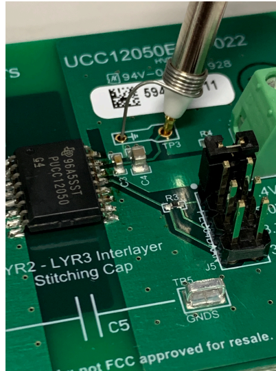
Figure 4. Using the pig tail test points: TP1, TP2, TP3
