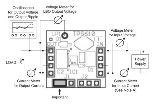
Note A: Use this current meter only if the sense wires of the supply are used.
