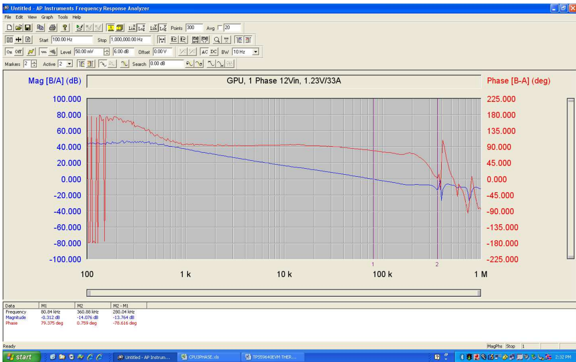
Figure 71. GPU Bode Plot at 12Vin, 1.23 V/33 A
