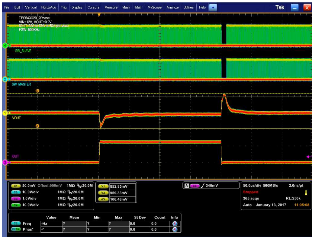
Figure 7. Transient Response of 0.9-V Output at 12 V IN , Transient is 25 A to 50 A, Step is 25 A at 30 A/μs
