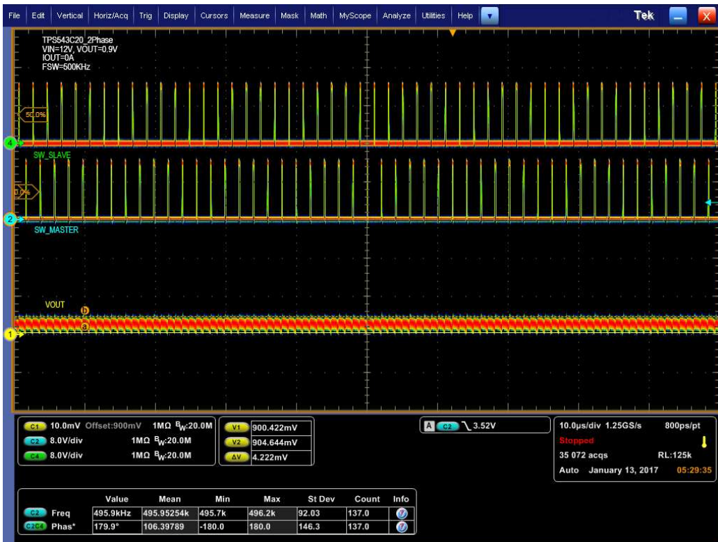
Figure 11. Output Ripple and SW Node of 0.9-V Output at 12 V IN , 0-A Output
