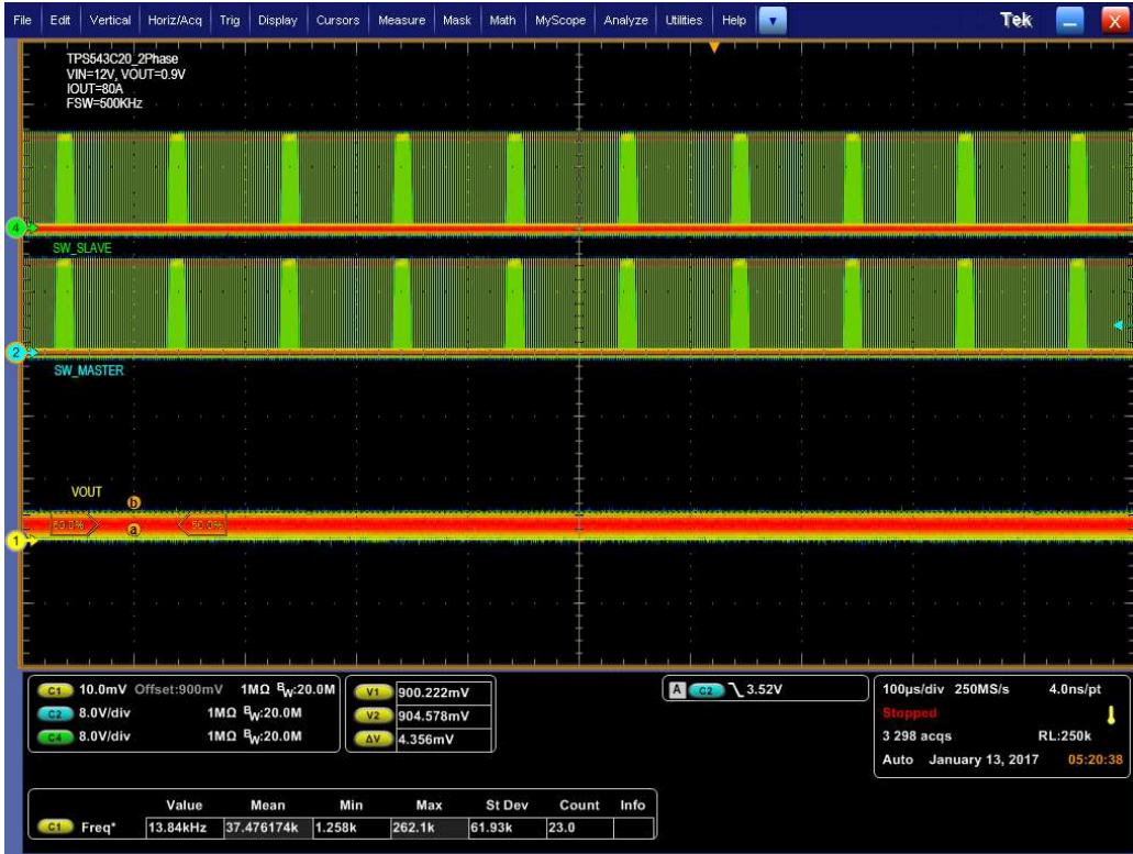
Figure 10. Output Ripple and SW Node of 0.9-V Output at 12 V IN , 80-A Output
