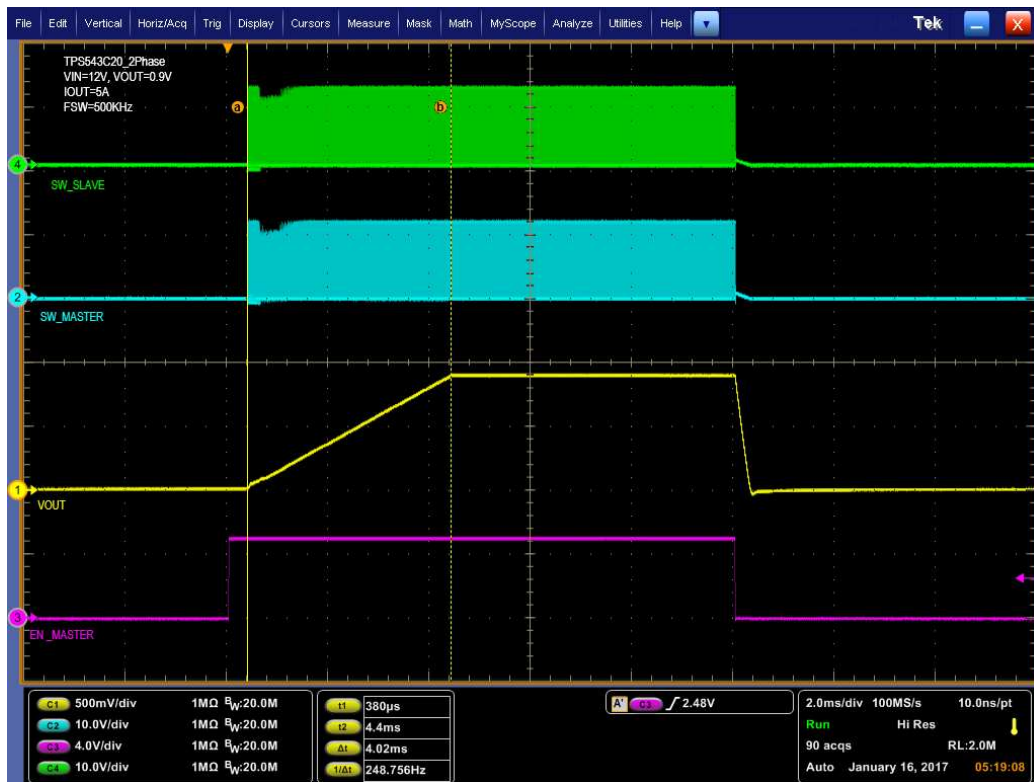
Figure 14. Output Voltage Start-up and Shutdown, 0.9-V Output at 12 V IN , 5-A Output
