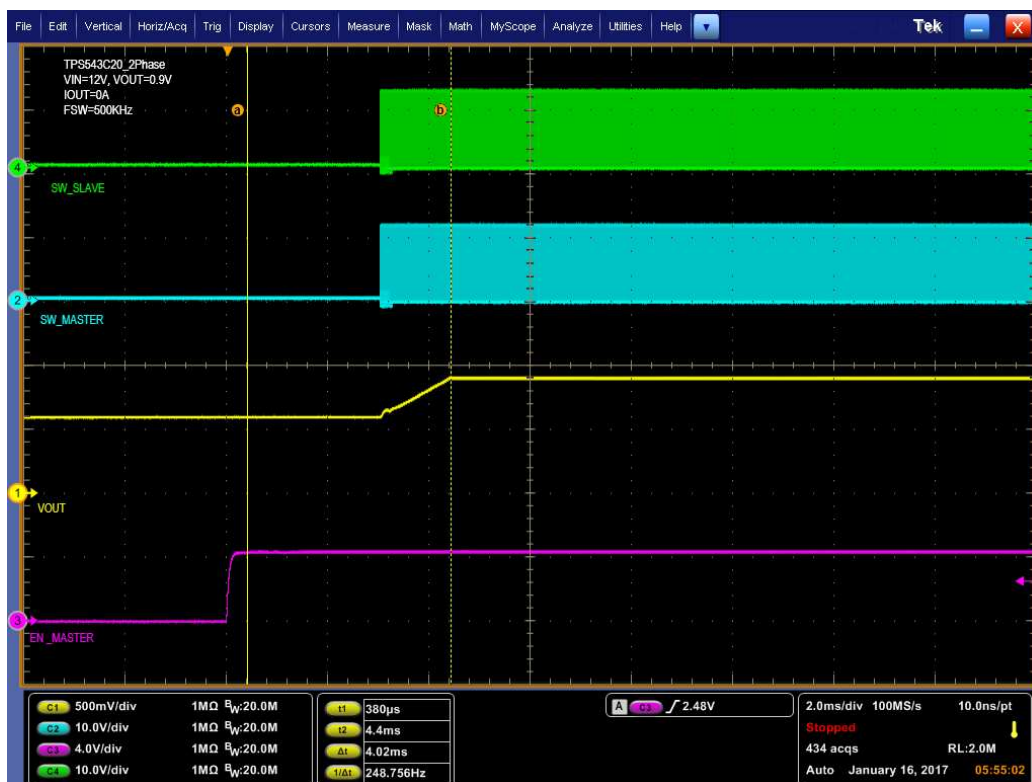
Figure 13. 0.6-V Pre-Bias Start Up From Enable, 0.9-V Output at 12 V IN , 0-A Output
