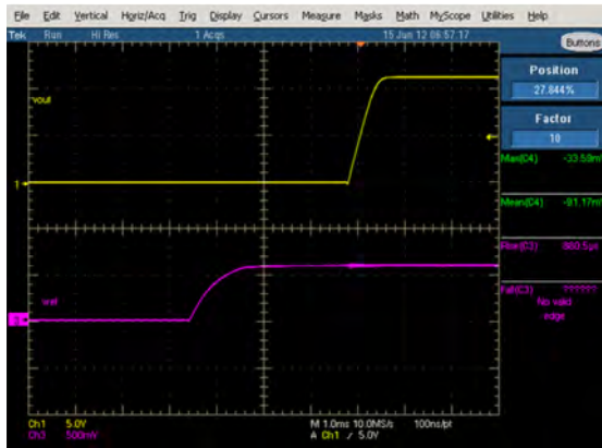
Figure 1. Vref and Vout start-Up Vin=48V Vo=12V
