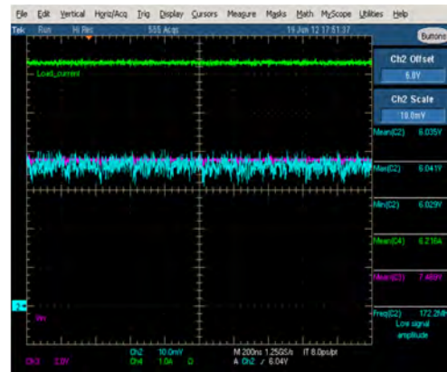
Figure 32. Ripple 8Vin Vo=6V, 6A 5MHz
