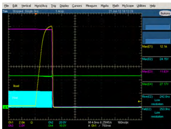
Figure 17. Current limit operation R_{ds\_on} = 13 \text{ m}\Omega , R_{lim} = 128 \text{ k}\Omega Ch1 (yellow): output current, Ch2 (blue): switching node Ch3 (purple): output voltage, Ch4 (green): input voltage
