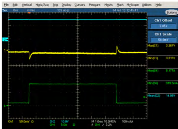
Figure 37. Transient step response Vin=15V, Vo=3.3V 2.2MHz 1-8A
