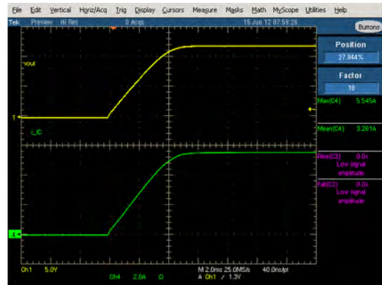
Figure 2. SS Vin=24V, Cref=1nF, CVdr=1μF, Cv3V=1μF, css=68nF, Io=5.5A
