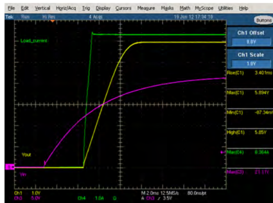
Figure 4. Start-up 22Vin Vo=5.8V, 6A, 5MHz
