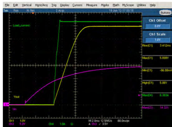
Figure 3. Start-up 15Vin Vo=5.8V, 6A, 5MHz
