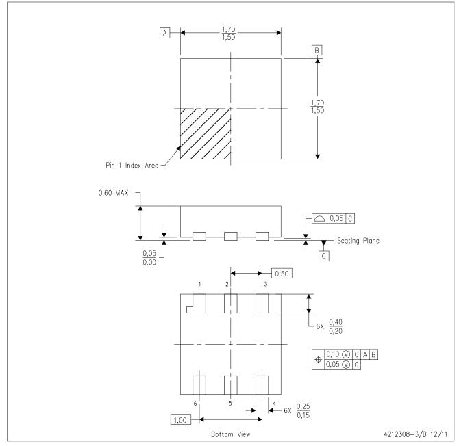
A. All linear dimensions are in millimeters. Dimensioning and tolerancing per ASME Y14.5M-1994.
