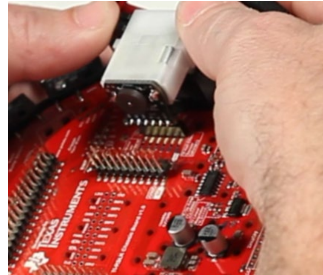
Figure 9. Ensure the motor is straight and pins are aligned before pressing down firmly.
