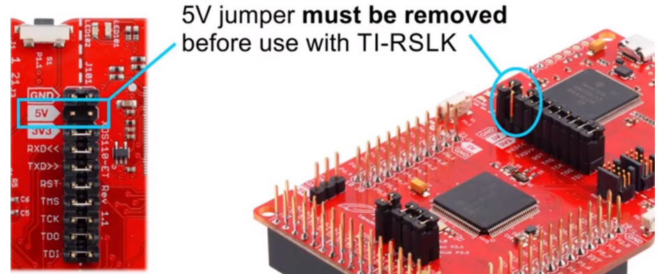
Figure 20. MSP432P401R LaunchPad with 5V jumper removed
