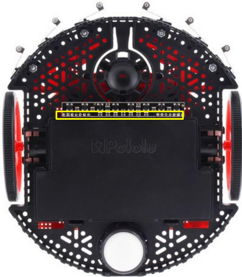
Figure 18. Insert the QTRX sensor with the largest part of the board facing the front of the robot
