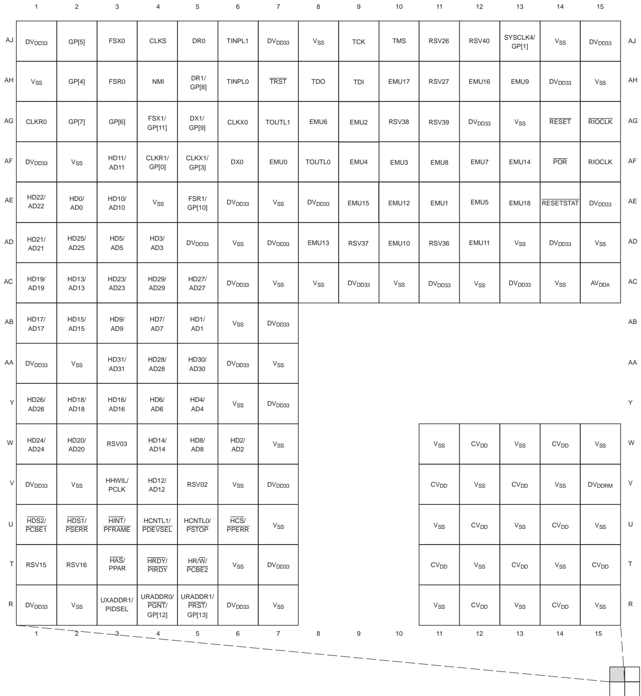
Figure 2-2. C6455 Pin Map (Bottom View) [Quadrant A]
