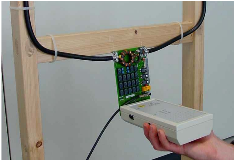
Figure 16: Tuning procedure at the base antenna
