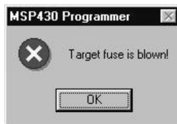
Figure 2–3. Communication Error Box for Blown Fuse
