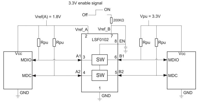
Figure 9. Typical Application Circuit (MDIO/Bidirectional Interface)
