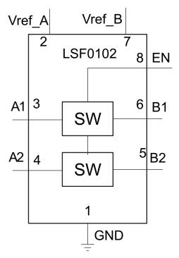
Figure 4. LSF0102 Functional Block Diagram
