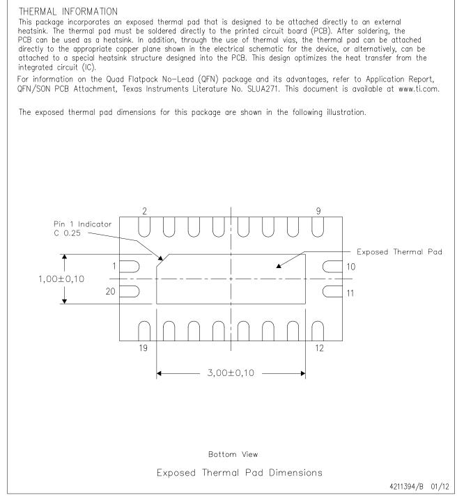
NOTE: All linear dimensions are in millimeters
