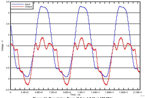
Figure 11. Translation Down (3.3 to 1.8 V) at 150 MHz
