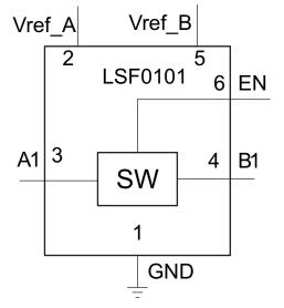
Figure 3. LSF0101 Functional Block Diagram
