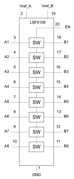
Figure 5. LSF0108 Functional Block Diagram
