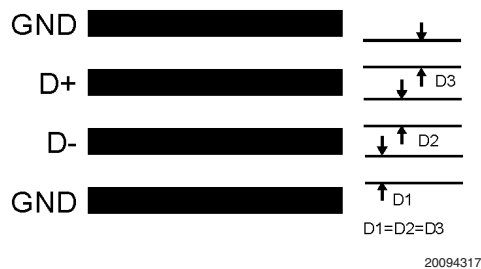
FIGURE 4. Ideal Diode Trace Layout
