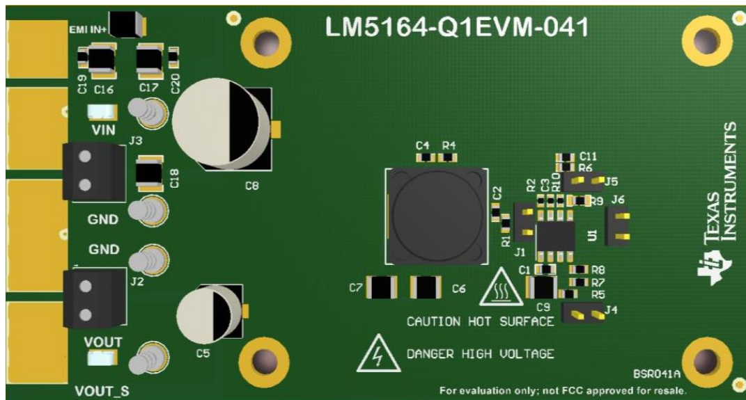
Figure 3. LM5164-Q1 EVM Top View
