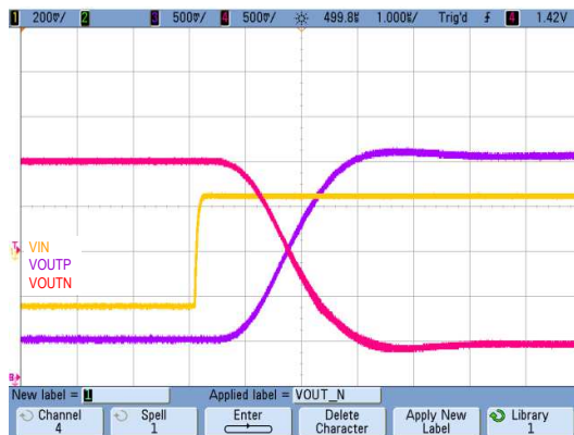
Figure 50. Step Response of the AMC1301 Device
