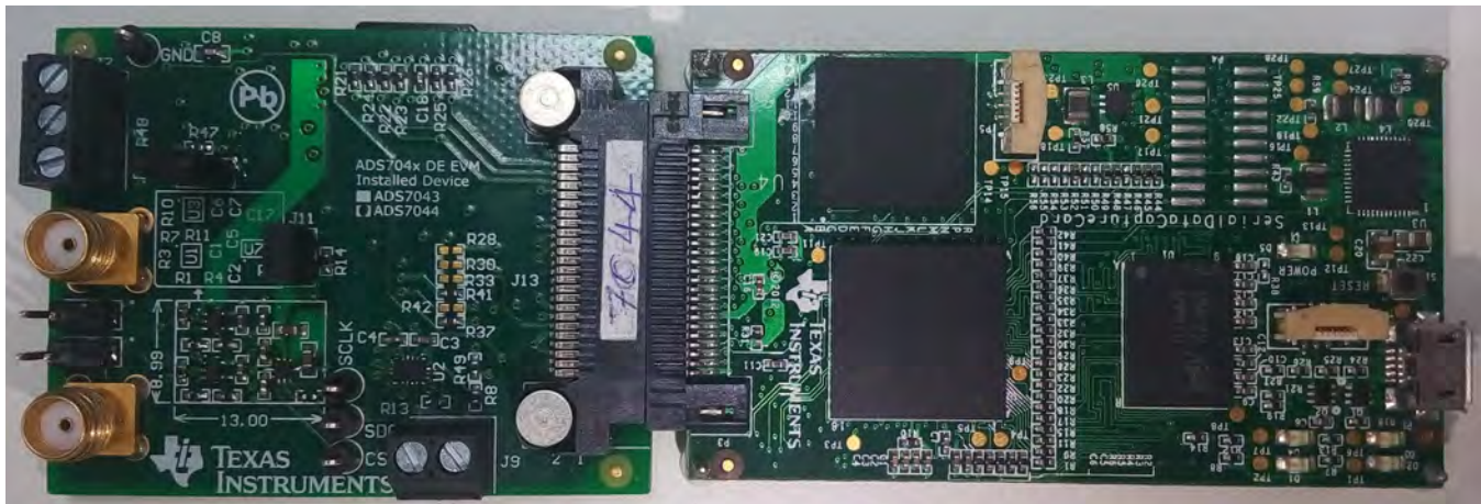
Figure 5. Connecting ADS7044EVM Board to Simple Capture Card
