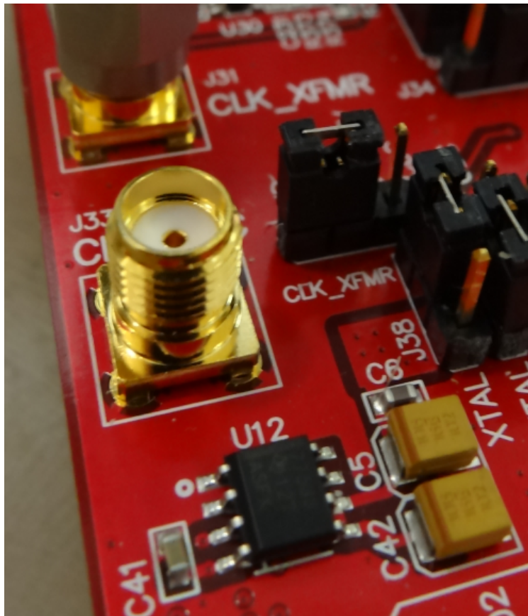
Figure 37. Jumper J35 and J38 positions for Disabled XTAL
