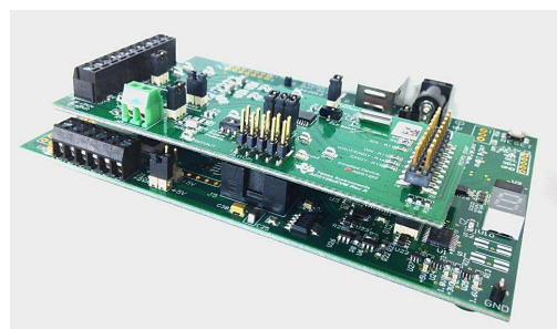
Figure 2. ADS126xEVM connected to MMB0 motherboard
