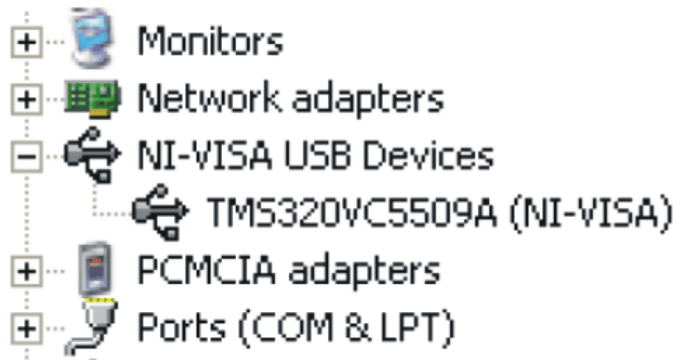
Figure 20. NI-VISA Driver Verification Using Device Manager
