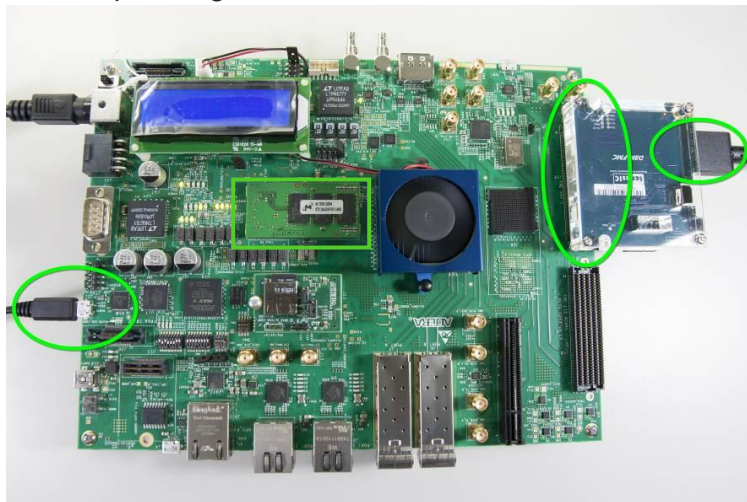
Figure 5-8 Setup A10SoC_D8M_FMC_VIP demonstration
