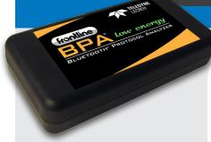
The Frontline BPA low energy Protocol Analyzer includes powerful Frontline software and the BPA low energy hardware interface.
