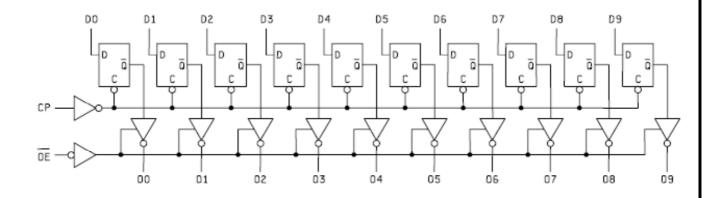
FIGURE 3. Logic diagram.
