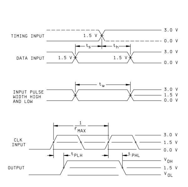
FIGURE 5. Switching waveforms and test circuit.
