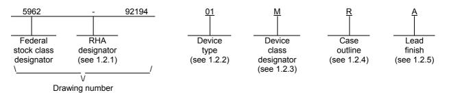
1.2.1 <u>RHA designator</u>. Device classes Q and V RHA marked devices meet the MIL-PRF-38535 specified RHA levels and are marked with the appropriate RHA designator. Device class M RHA marked devices meet the MIL-PRF-38535, appendix A specified RHA levels and are marked with the appropriate RHA designator. A dash (-) indicates a non-RHA device.
