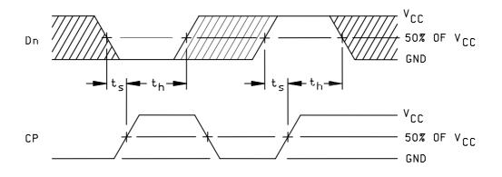
FIGURE 4. Switching waveforms and test circuit.
