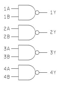
FIGURE 3. Logic diagram.
