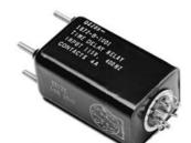
CII 1600/1700 series delay on operate timers combine solid state timing circuits with electromechanical output relays in robust hermetically sealed enclosures. The 1600 types are fixed timers, while the 1700 models are adjustable via an external resistor. Numerous output options include 4A rated
