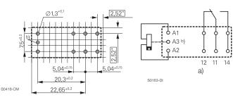
\*) With the recommended PCB hole sizes a grid pattern from 2.5mm to 2.54mm can be used.
