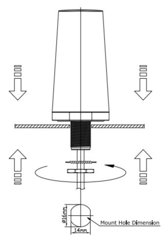
Recommended torque for mounting is 4.018 N.m or 41 kgf.cm Maximum torque for mounting is 9.8 N.m or 100 kgf.cm
