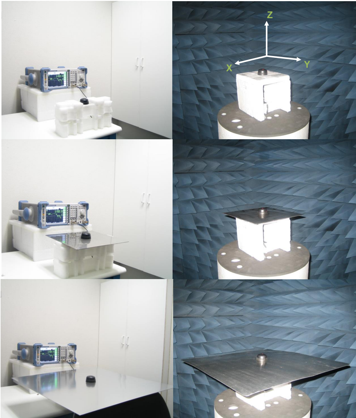
Figure 1. G21 Antenna test set up in free space, 30x30 cm metal plate and 60x60 cm metal plate, R&SZVL6 VNA (left) and R&S4100 CTIA 3D Chamber (Right).
