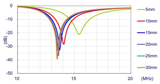
The minimum distance of the antenna placement away from metal is 15mm recommended.
