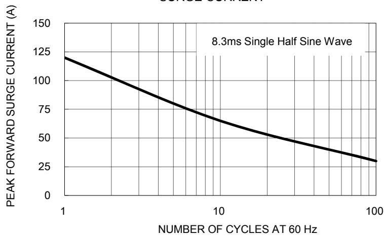
FIG. 3 MAXIMUM NON-REPETITIVE FORWARD SURGE CURRENT
