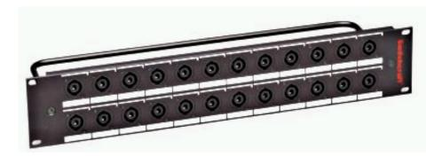
The HPC Loudspeaker Patchbay features a 19 rack unit loaded with HPC loudspeaker connectors. Available with either 0.250 Faston terminals or 0.187 Faston terminals. One rack unit height versions come with 12 HPC loudspeaker connectors, two rack unit height versions come with 24 HPC loudspeaker connectors. All versions have a rugged cable tie bar, which takes the weight of the cabling away from the connections.
