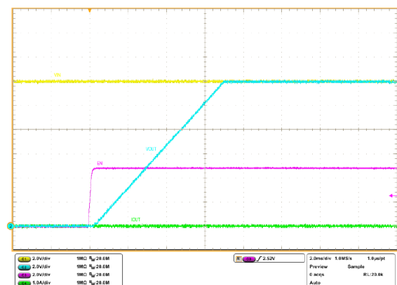
Figure 23. Start-up via En/Fault pin (No load)
