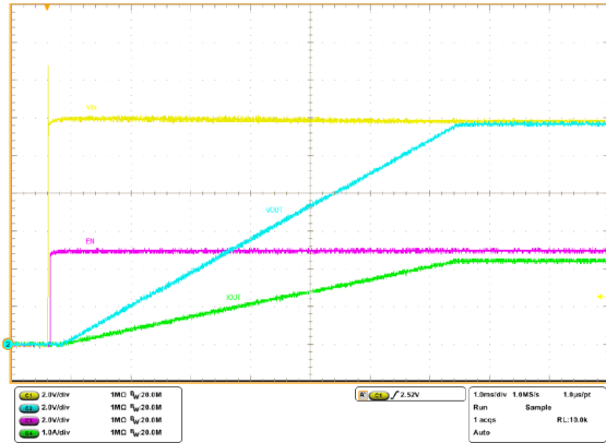
Figure 24. Start-up via input voltage (5 Ω load)
