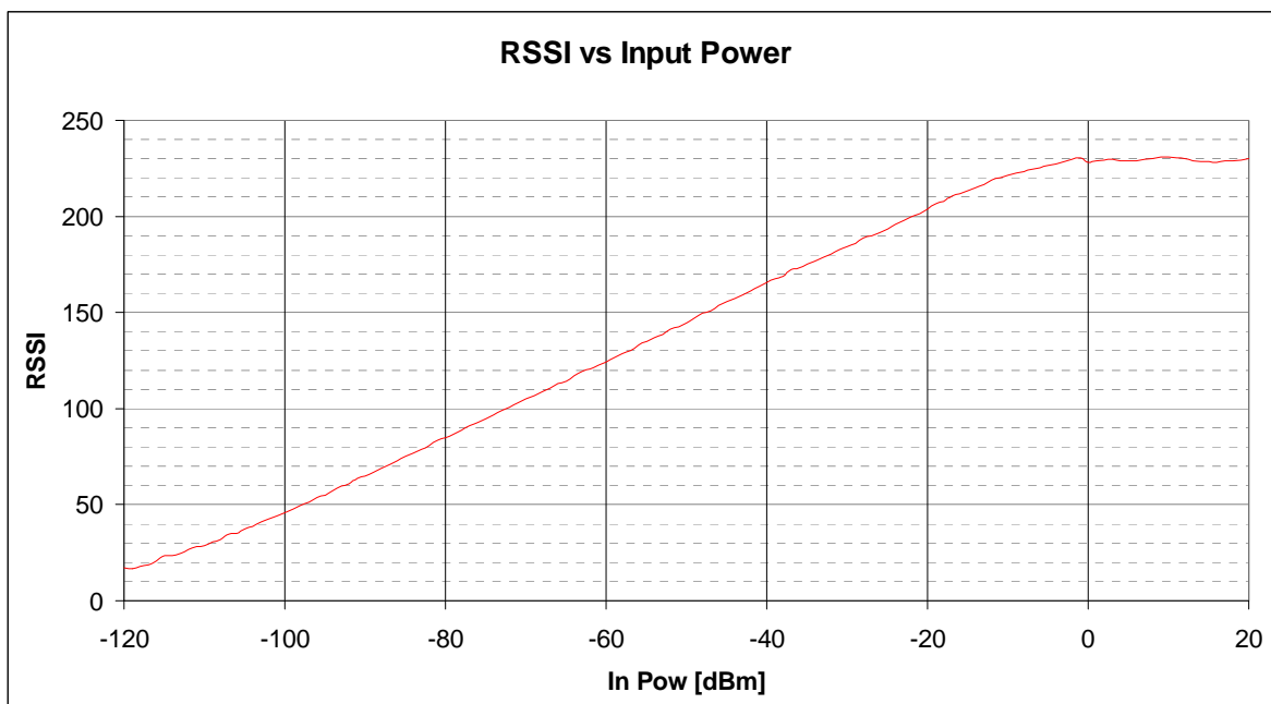
Figure 32.25. RSSI Value vs. Input Power
