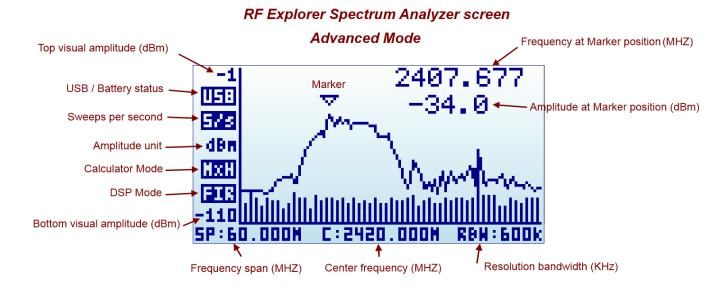
Note the frequency axis indicators changes at the bottom. More details about this screen mode in section *Analyzer screen* page 18.
