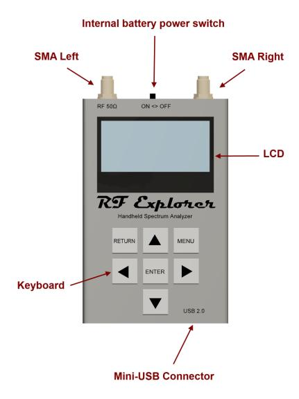
The RF Explorer Standard models includes 7 functional buttons in the front side. The unit also includes at least one RF connector 50 ohm impedance standard SMA format.
