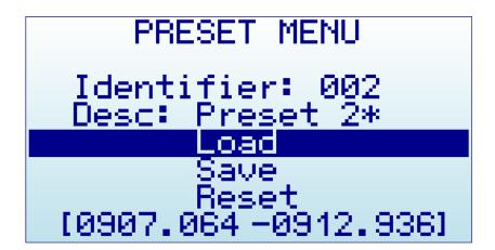
Preset is a convenient facility to store multiple configurations which can be easily recovered. This feature is supported in selected models only: RF Explorer Combo models (since firmware v1.26) and RF Explorer Plus models.
