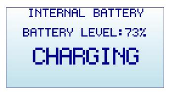
At this point you can close this screen pressing ENTER or RETURN. If you keep it active for more than 15 seconds, it automatically sets the device in SLEEP MODE - all internal circuits and LCD backlight go off, except for charging and minimal CPU monitoring - This is the recommended procedure to charge the device
