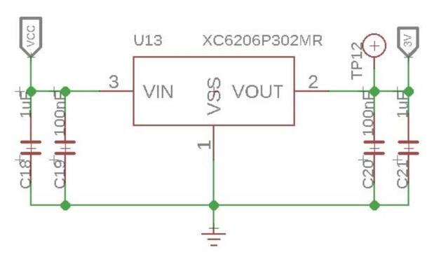
The operating voltage range of BMI088 is 2.4-3.6V, so we use the XC6206P30 chip to provide a stable 3.0V. The input of XC6206P30 ranges from 1.8V to 6.0V, so you can use this module with your Arduino both in 3.3V and 5V.
