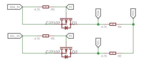
This is a typical Bi-directional level shifter circuit to connect two different voltage section of an I<sup>2</sup>C bus. The I<sup>2</sup>C bus of this sensor use 3.3V, if the I<sup>2</sup>C bus of the Arduino use 5V, this circuit will be needed. In the schematic above, **Q1** and **Q2** are N-Channel MOSFET CJ2102, which act as a bidirectional switch. In order to better understand this part, you can refer to the AN10441
