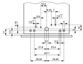
D1 = 6.2 mm mounting from above / D1 = 3.6 mm mounting from below PC Board 1.6 mm / Dimensions without tolerance:  $\leq$  15 =  $\pm$  0.05 / > 15 =  $\pm$  0.10 Drilling diagram CMF4 and CMF5 mirror-inverted
