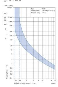
The above tripping characteristics apply to symmetrical overloads on the two poles.
