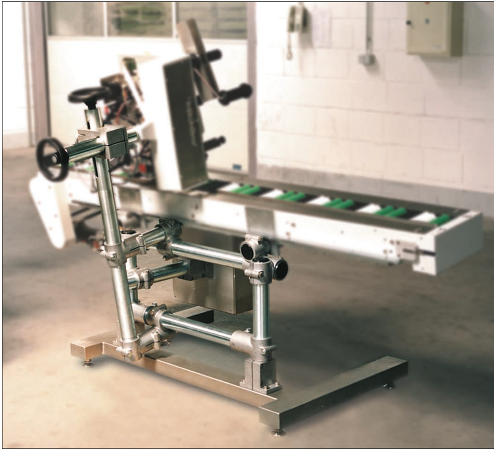
Frame for a labelling machine.
