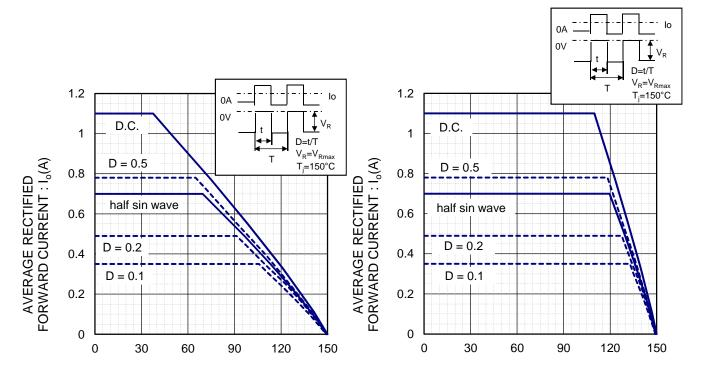
$\begin{aligned} & \text{AMBIENT TEMPERATURE} : T_a(^\circ\text{C}) \\ & \text{DERATING CURVE} \; (I_o\text{-}T_a) \end{aligned}$
