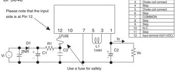
Verify proper operation under actual conditions before use. In particular, confirm that the load current does not exceed the maximum rating.
